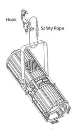
• Please use qualified safety-rope, which can hold at least 10 times the weight of the fixture. You must only use safety-ropes with quick links with screw cap. Pull the safety-rope through the hole on the bottom of the base and over the trussing system etc. Insert the end in the quick link and tighten the fixation screw. A safety rope which already hold the strain of a crash or which is defective must not be used again.
